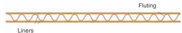
Corrugated board structure
